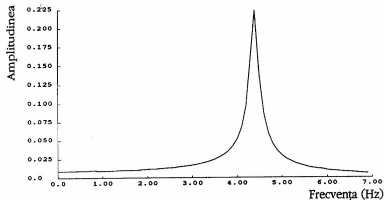
Figure 4. Resonance amplitude for the top of the tower due to wind excitation
