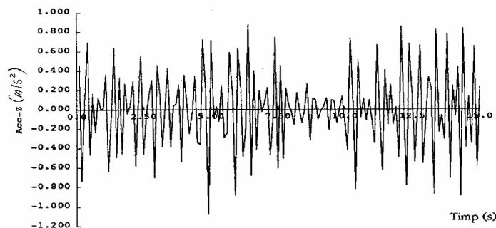
Figure 10. Time history in acceleration of the top of the tower in global direction Z shows a maximum acceleration of 0,12g.
