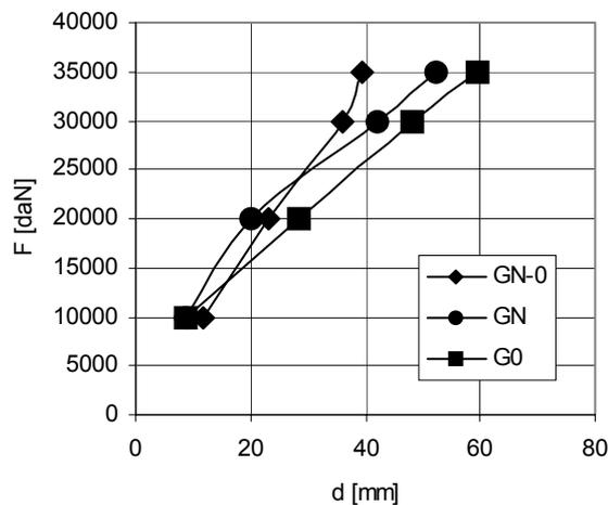
Fig. 12 The maximum displacements for the 3 tested beams
