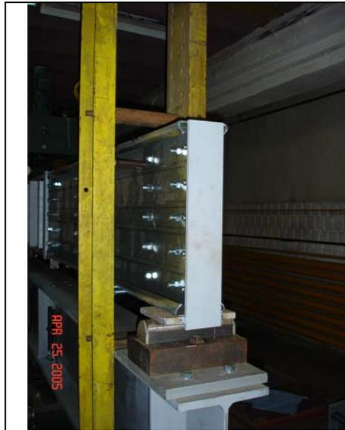
Fig. 9 The driving elements mounted to prevent the lateral buckling
