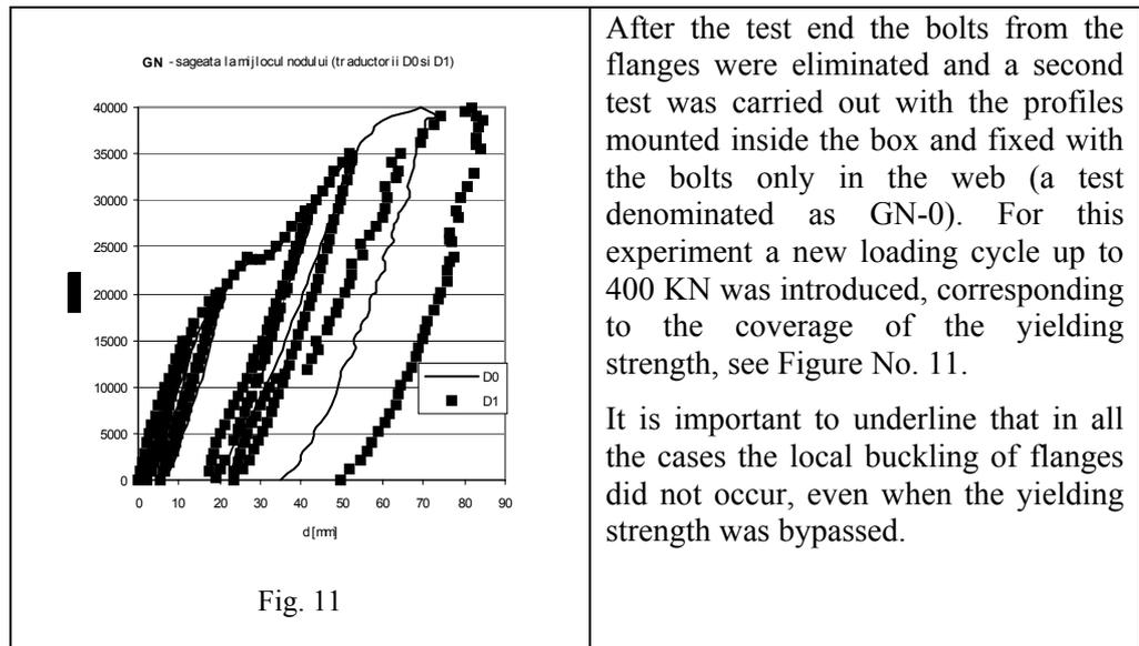
After the test end the bolts from the flanges were eliminated and a second test was carried out with the profiles mounted inside the box and fixed with the bolts only in the web (a test denominated as GN-0). For this experiment a new loading cycle up to 400 KN was introduced, corresponding to the coverage of the yielding strength, see Figure No. 11.
