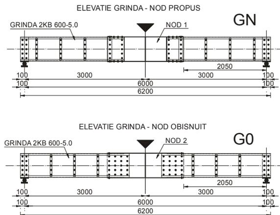
Fig. 6 The dimensions of the proposed specimens
