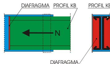
Fig. 3 Steel plate that undertakes the axial force
