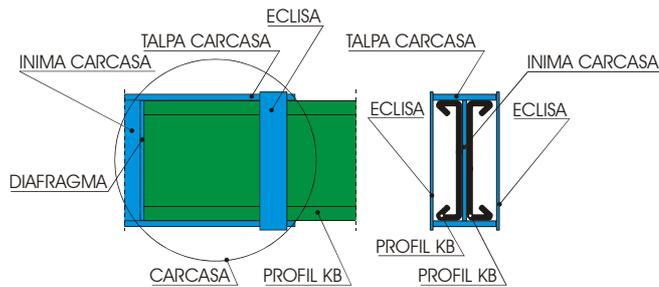
Fig. 2 Box-type joint
