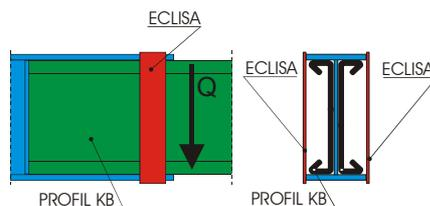
Fig. 4 Steel plate to undertake the shear
