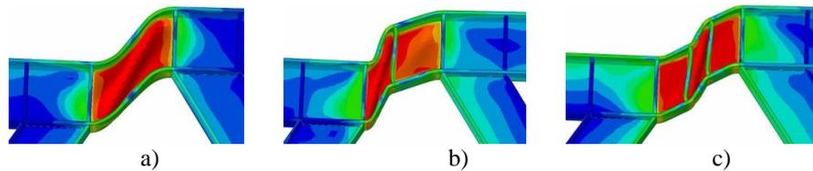
Figure 8. Deformed shapes of the link elements at the end of analysis:
