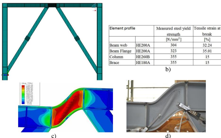
Figure 3. a) Mesh of the finite element EBF model; b) material characteristics used in calibration; The deformed shape of the dissipative link elements: c) FE Model d) Laboratory test
