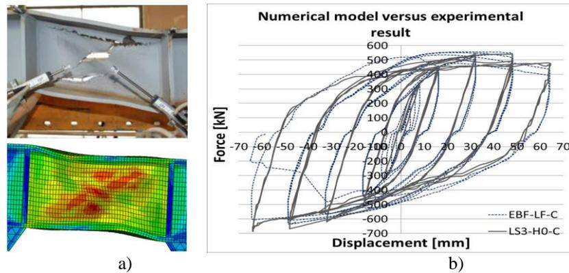
Figure 12. a) Deformed shape of the link element at the end of experimental testing of specimen EBF-LF-C; b) Force-displacement calibration curve-experimental versus numerical response.
