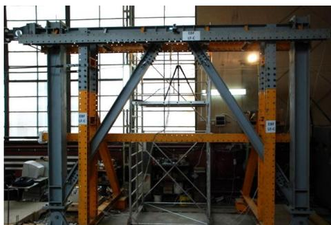
Figure 2. a) Force-displacement curve for steel EBF; b) Shear force-rotation curve of dissipative element; c) Experimental set-up
