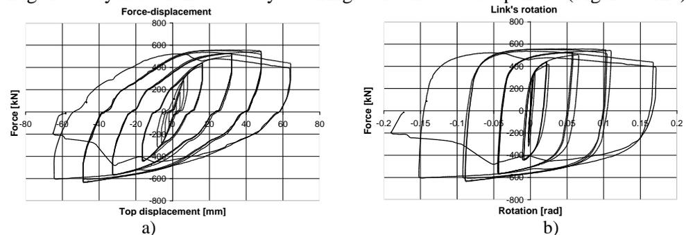
Figure 11. a) Force-displacement curve; b) Shear force-rotation curve.
