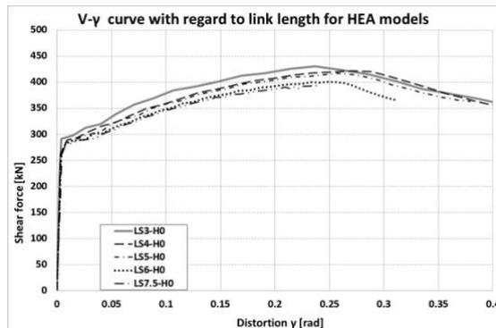
Figure 5. Shear force-distortion curve for different link lengths
